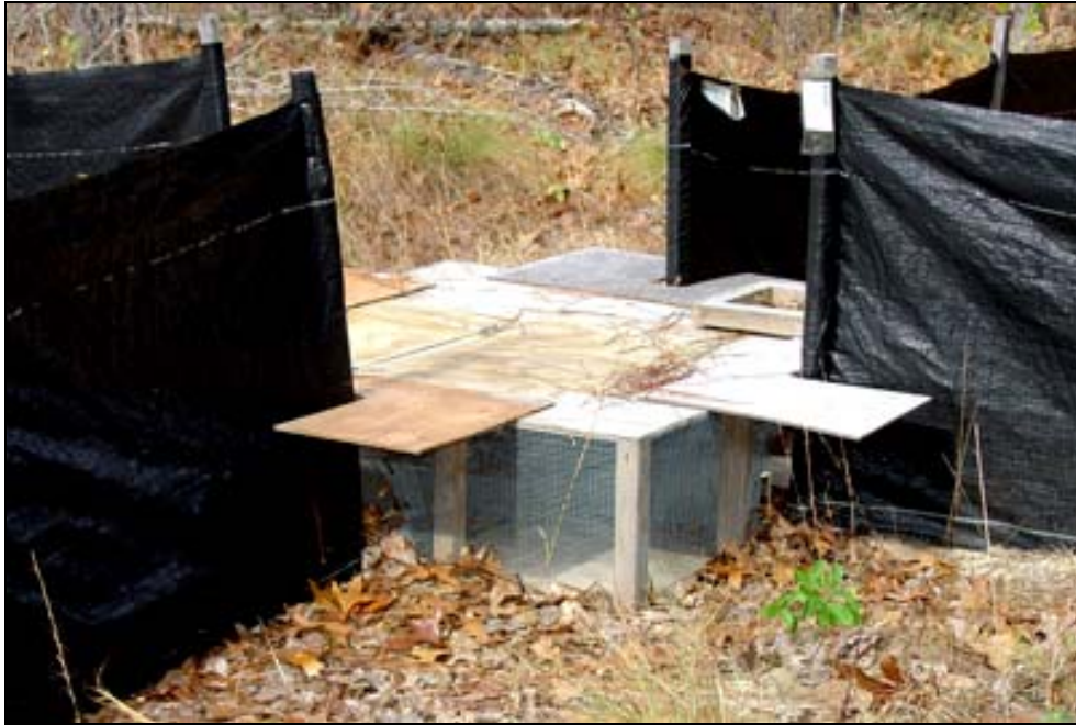
Figure 4.1. Trap used for Drymarchon couperi , 2002–2003, Georgia. Photo highlights the horizontal panels (0.75 m x 0.75 m) extending over each funnel entrance into the box trap.
